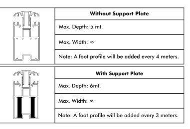
Thanks to Adjustable Roof Angle Adjustment Profile Roof Gutter Profile and Wall Fixing Profile **Provides 0-22 Degree Angle**
